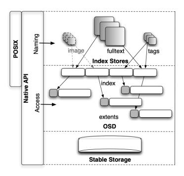
Figure 1: **hFAD Architecture** Index stores combined with arbitrary-length extents provide the primary means of accessing stable storage. A POSIX interface can easily be implemented on top of these services.
