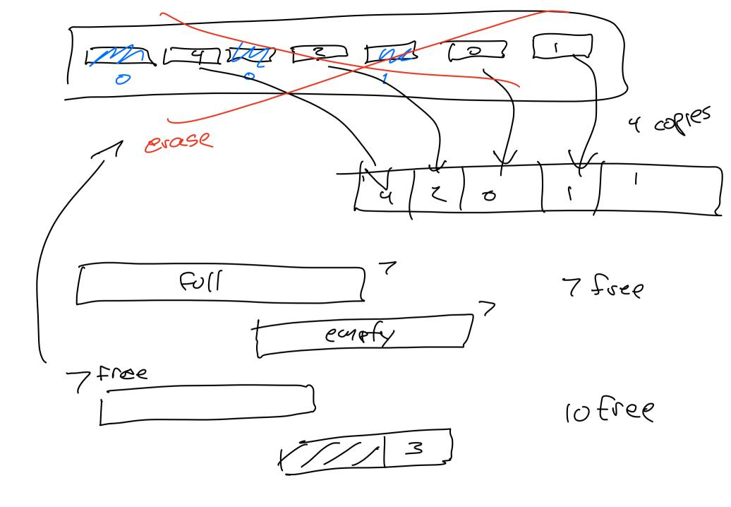
Write amplification! sufernal flash write ops = "real" writes (from comporter) + GC writes (moving data so can) evase a unit) higher write aurp. If! - random small writes - low free space % TRIM -> tell SSD to forget blocks ust (discard) used by file system
