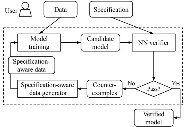
**Figure 2.** OUBOROS’s workflow. The dotted frame is OUBOROS system. Users provide data and specifications and receive verified models that satisfy the specifications.
