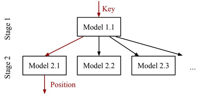
**Figure 1.** A two-stage Recursive Model Index (RMI). In this example, this RMI takes a “Key” as an input, chooses “Model 1.1” and “Model 2.1” for prediction, and finally produces the “Position” which is supposed to be the data location indexed by “Key” in the database.
