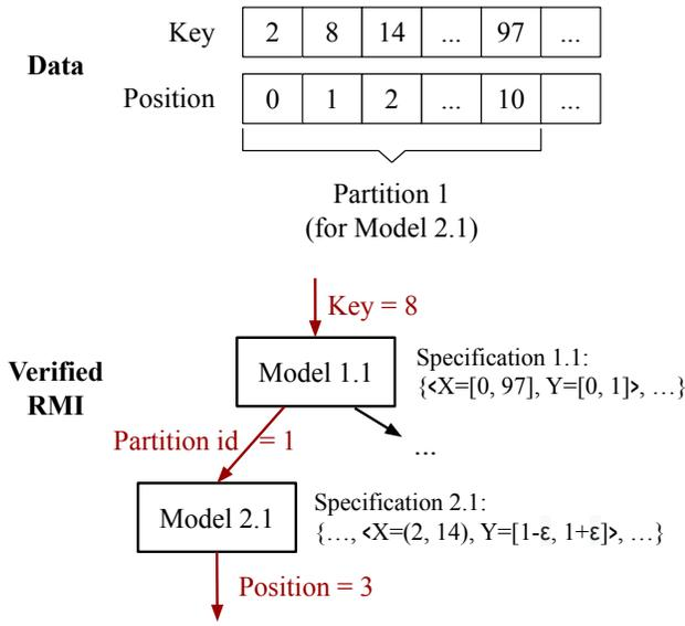
**Figure 3.** An example of a RMI. On the top is the (sorted) data that the RMI indexes. On the bottom is a verified two-staged RMI with specifications for each model. In this example, the RMI predicts that the data indexed by “Key=8” should locate at “Position=3”, and the true position is “1” (see “Data”). If the user-defined error bound is less than 2 ( $\epsilon < 2$ ), this RMI will be rejected by NN-verification because “Model 2.1” does not satisfy “Specification 2.1”.
